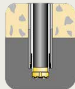
4. Drilling continues to the desired depth in the bedrock using a conventional drillstring.
