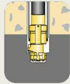
1. When drilling starts, the ODEX reamer swings out and reams the pilot-hole wide enough for the casing tube to slide down behind the drill bit assembly.
