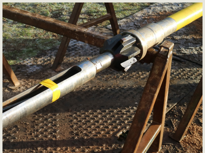
Umbilical connected and secured in the lifting sub eye
