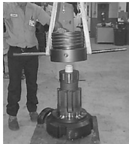
QL200 - Removing chuck from bit
